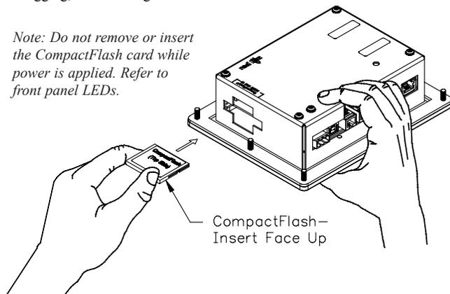
Information stored on a CompactFlash card by a 303 can be read by a card reader attached to a PC. This information is stored in IBM (Windows®) PC compatible FAT16 file format.
