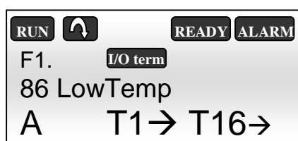
Figure 5.1-3, Low temperature alarm on the NXP panel
