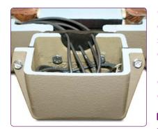
Oversized, gasketed conduit box with lead separation gasket and conduit box cover gasket restricts moisture and contaminants from entering the motor.
