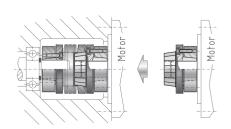
WITH CONICAL CLAMPING RING AND BLIND MATE CONNECTION
