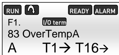
Figure 7.1-2, High temperature alarm on the NXP panel
