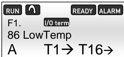
Figure 7.1-3, Low temperature alarm on the NXP panel
