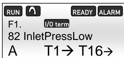
Figure 7.1-4, Low pressure alarm on the NXP panel
