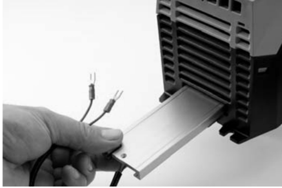
Figure D-2 Dynamic Braking Resistor Installation
