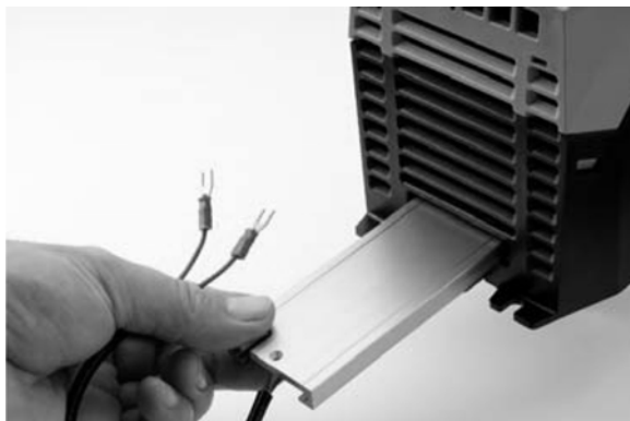
Figure D-2 Dynamic Braking Resistor Installation
