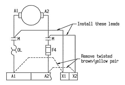
CAUTION: Armature overvoltage may occur when M contactor is opened at high speed without X1 and X2 reconnected as shown.
