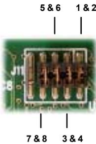
CAN (Controller Area Network) is a 1Mb/s local area network. Two CAN channels are supported by NextMove PCI - CANopen and Baldor CAN. Access to both channels is configured by a 10-pin 2mm pin header, J11, mounted along the top edge of the NextMove PCI card. Jumpers link pin pairs 1 and 2, 3 and 4, 5 and 6, 7 and 8. These jumpers route the CAN signals to the breakout module and only need to be removed if you are connecting a CAN Bracket card.
