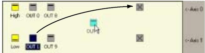
5. Click **Apply** at the bottom of the screen. This sends the output configuration to the NextMove PCI.
