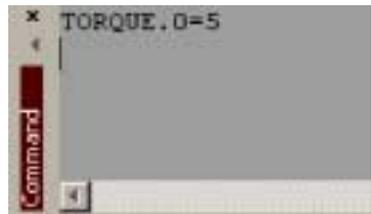
See section 4.3.2 for details of the demand outputs. In WorkBench v5, look at the Spy window located on the right of the screen. The virtual LED Command display should show 5 (approximately). If there seems to be no command output, check the electrical connections between the breakout module and the drive.
