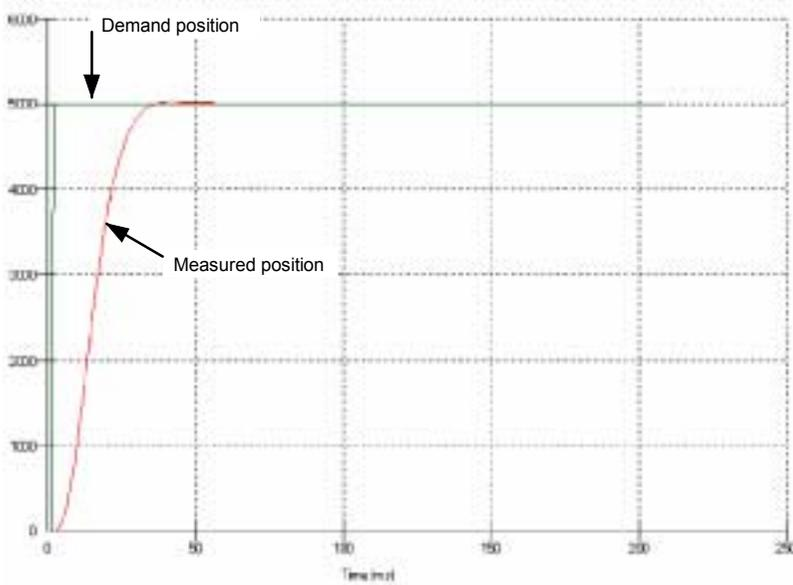
Figure 14 - Critically damped (ideal) response
