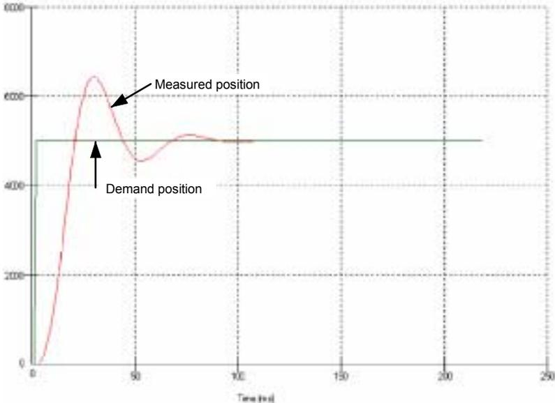
Figure 12 - Underdamped response
