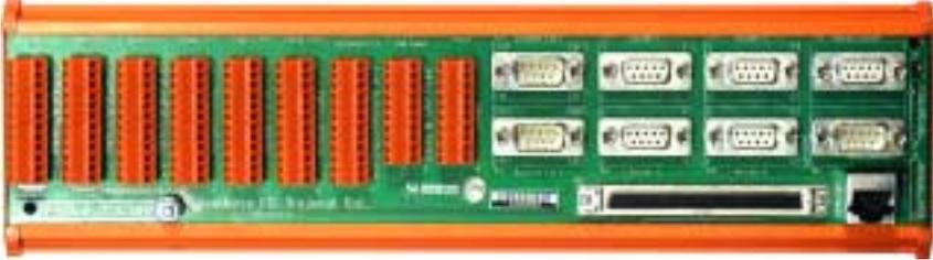
**Figure 18 - NextMove PCI Breakout module**
