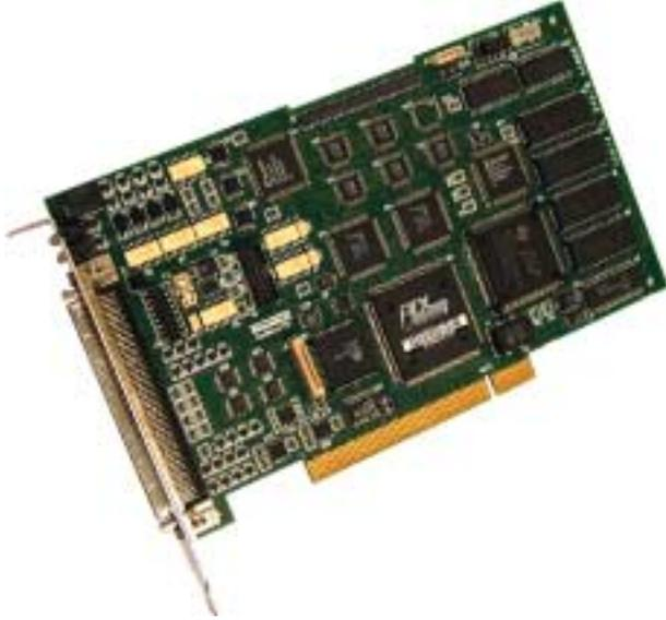
NextMove PCI features the MintMT motion control language. MintMT is a structured form of Basic, custom designed for stepper or servo motion control applications. It allows you to get started very quickly with simple motion control programs. In addition, MintMT includes a wide range of powerful commands for complex applications.
