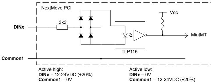
Figure 4 - Digital input circuit - fast interrupts
