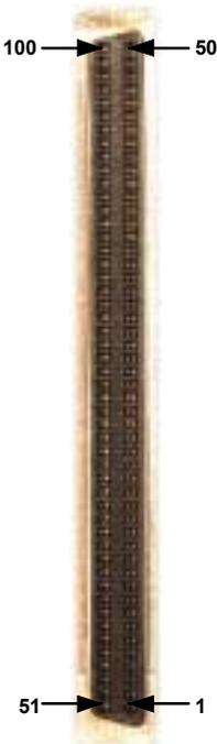
The pin assignment for the 100-pin D-type connector is shown in Table 1.
