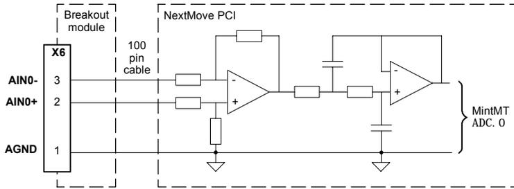
**Figure 1 - Analog input wiring, AIN0 shown**
