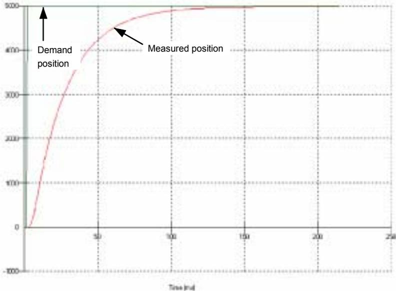
Figure 13 - Overdamped response
