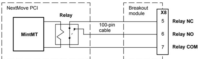
Figure 8 - Relay connections
