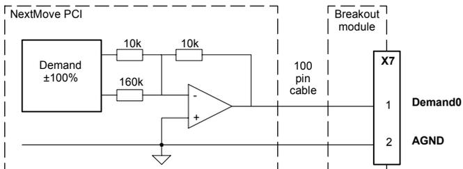
Figure 2 - Analog output circuit - Demand0 shown
