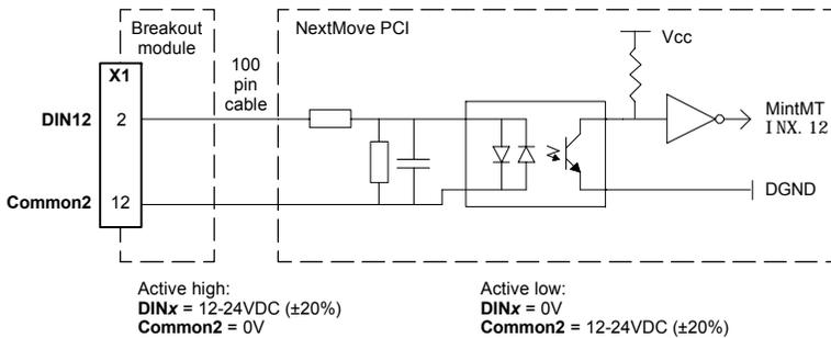
Figure 3 - Digital input circuit - DIN12 shown
