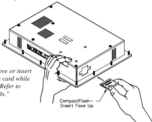
*Note: Do not remove or insert the CompactFlash card while power is applied. Refer to "Front Panel LEDs."*
